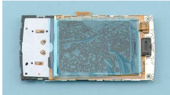
32) Protect the LCD with protective film.
