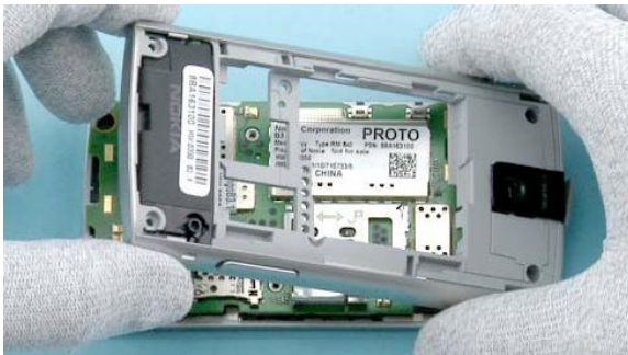
11) Release the D-COVER ASSY as shown.
