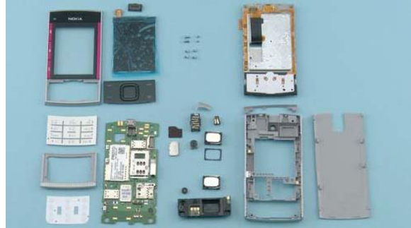
38) Nokia X6 disassembly is now complete.
