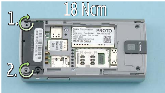
3) Tighten the two TORX+ size 6 screws to the torque of 18 Ncm in the order shown.
