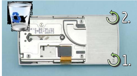
28) Make sure the slide is positioned as shown in the picture. Unscrew the two TORX+ size 5 screws in the order shown. Do not use them again. Discard them.
