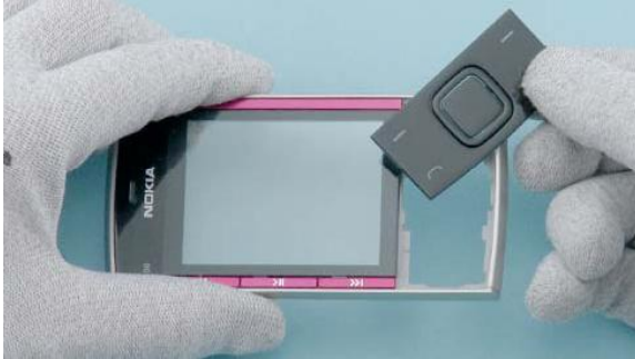
37) Separate the FUNCTION KEYMAT ASSY from the A-COVER ASSY.
