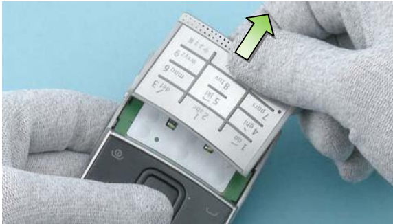
7) Remove the NUMERIC KEYMAT ASSY and the E-COVER ASSY as shown.
