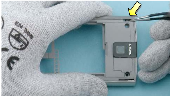
19) Use the tweezers to carefully release the clip holding the SPEAKER OUTL TRIM TOP ASSY.
