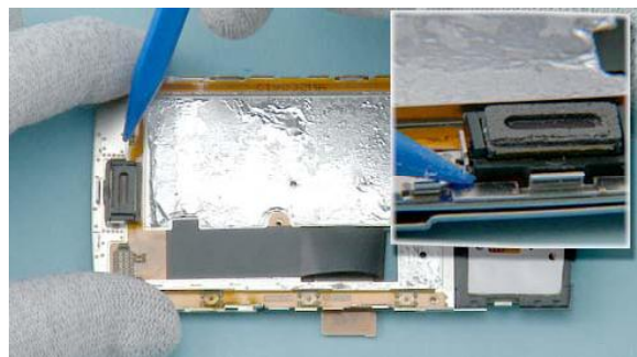
36) Use the sharp end of the SS-93 to release the EARPIECE. Remove the EARPIECE with the tweezers.
