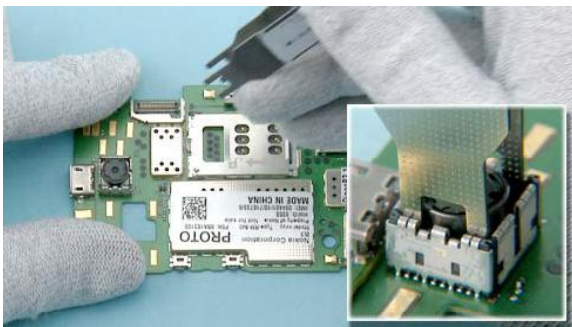
17) Use the camera removal tool SS-88 to detach the CAMERA.
