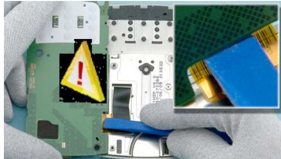
14) Disconnect the UI FLEX connector with the SS-93. Be careful not to damage the connector or any nearby components.
