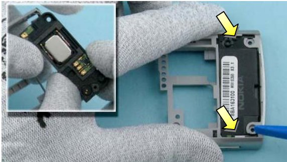
25) Use the SS-93 to release the ANTENNA MODULE. Press the ANTENNA MODULE lightly through the D-COVER.
