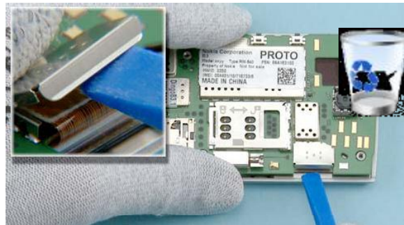
12) Use the SS-93 to carefully lift up the board to board connector SHIELD LID. The board to board connector SHIELD LID has to be always renewed.
