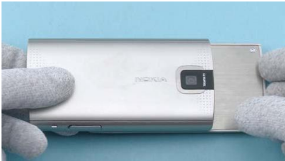
3) Slide the phone open and release the battery cover.
