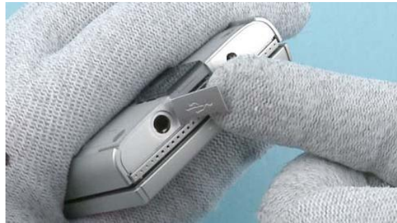
10) Before removing the D-COVER ASSY, open the USB DOOR.
